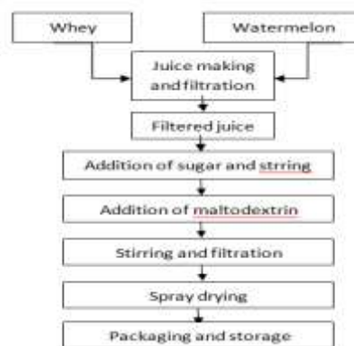
Figure 1: Process flow diagram for the whey melon preparation
