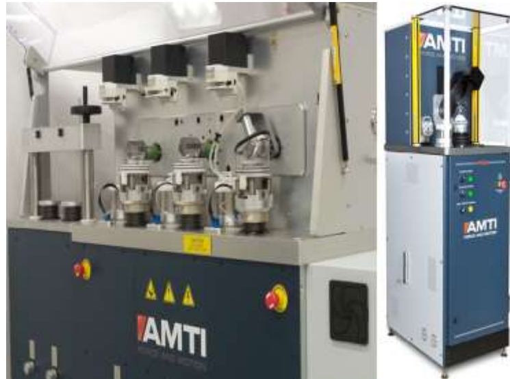
Fig 4.2 The AMTI wear test system has been the business standard for estimating knee wear (left). All the more as of late, progressed wear test systems like the AMTI VIVO give expanded stacking adaptability to evaluate more modern stacking conditions.
