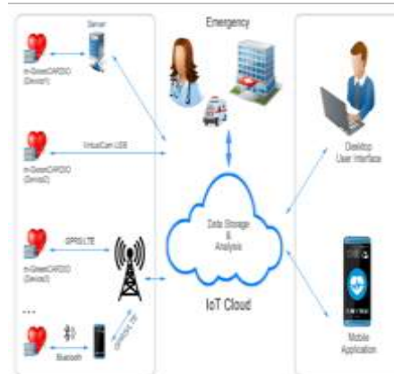
Fig 1: IoT based ECG Monitoring network (Source: https://www.researchgate.net/figure ).
