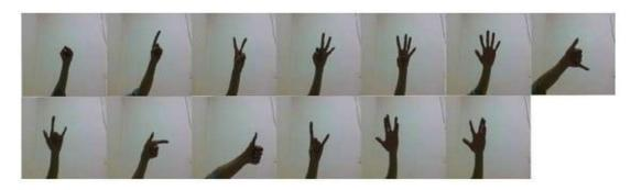
When the fingers are detected and recognized, the hand gesture can be recognized using a simple rule classifier. In the rule classifier, the hand gesture is predicted according to the number and content of fingers detected. The content of the fingers means what fingers are detected. The rule classifier is very effective and efficient. For example, if three fingers, that is, the middle finger, the ring finger, and the little finger, are detected, the hand gesture is classified.
