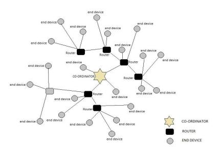
As given in the figure the clustered tree network is formed. The network joining is mainly based on the signal strength received at the co-ordinator and next its routers in a hierarchical order When the results are observed in the stimulated environment then the node connectivity graph has been improved over the previous DAAM protocol of ZigBee
