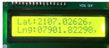
Fig.3 LCD displaying GPS coordinates
