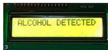
Fig.9 LCD display when alcohol is detected
