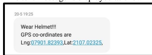
Fig.6 Text message when helmet is detected
