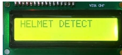
Fig.5 LCD display when helmet is detected
