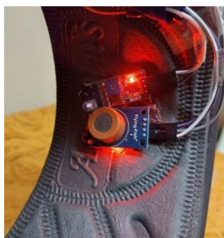
Fig.15 : Alcohol sensor and Helmet sensor mounted on Helmet
