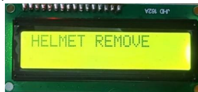
Fig.7 LCD display when helmet is removed
