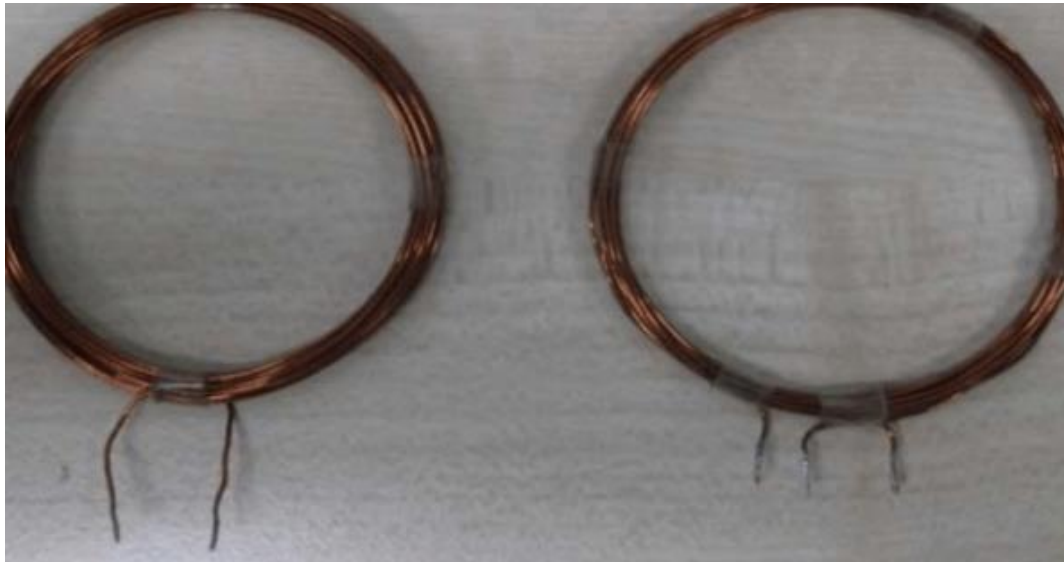
Figure. 3. Inductive Coupling in this case , as the antenna of Wireless Power Transfer
