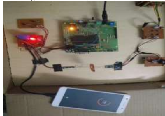
Fig. 9: Charging Phone using WPT
