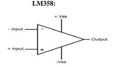
Op amp and comparator look very comparable but a comparator gives a logic output representing the comparative potentials on its two outputs. An op amp amplifies the discrepancy voltage between its two inputs and is planned always to be used in closed loop applications.
