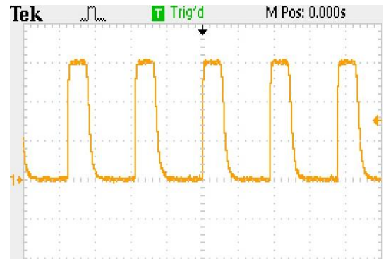
Figure 3.2(b): PWM pulse waveform at 31% duty cycle.
