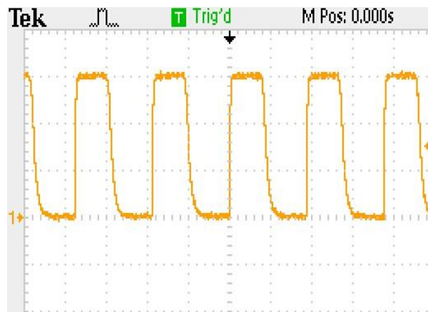
Figure 3.2(c): PWM pulse waveform at 46% duty cycle.
