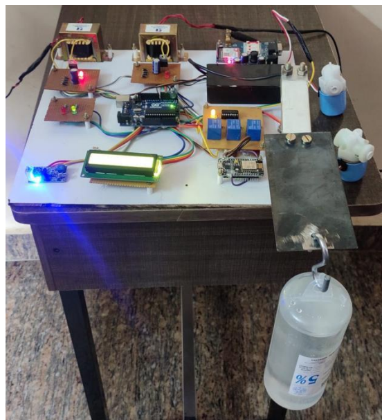
Fig 3: Position of saline placed in the load cell
