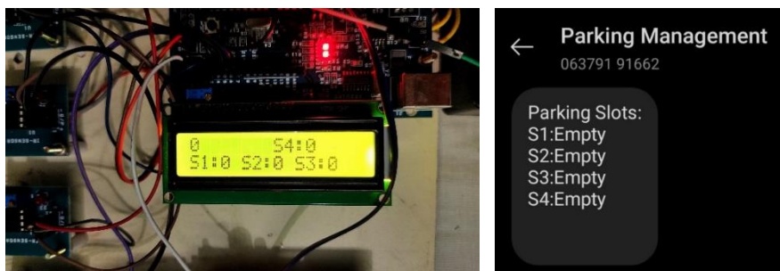
Fig.9.4 Parking slot empty condition
