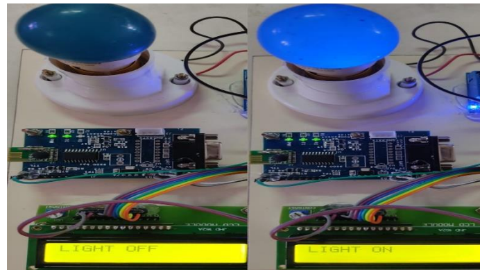
Fig 3.8 Home Automation Light ON and OFF
