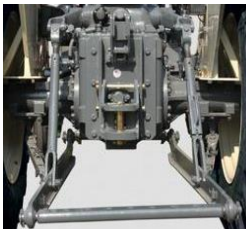
Fig 1 Existing Trailer Connecting Bed in Tractors
