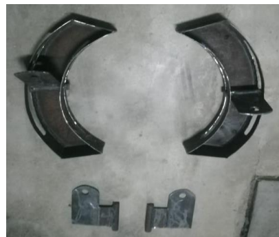
Fig 4 Fabrication of Anti-rolling Provision (ARP)
