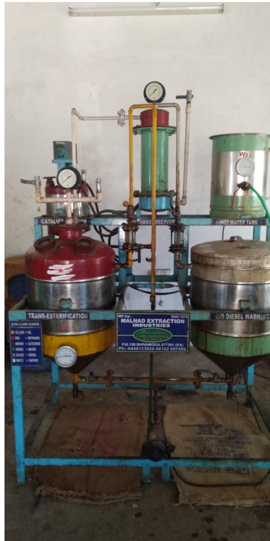
Fig.2: Equipment for Bio-diesel Production.
