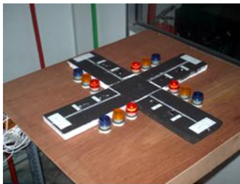
Fig 1.2 Traffic light hardware
