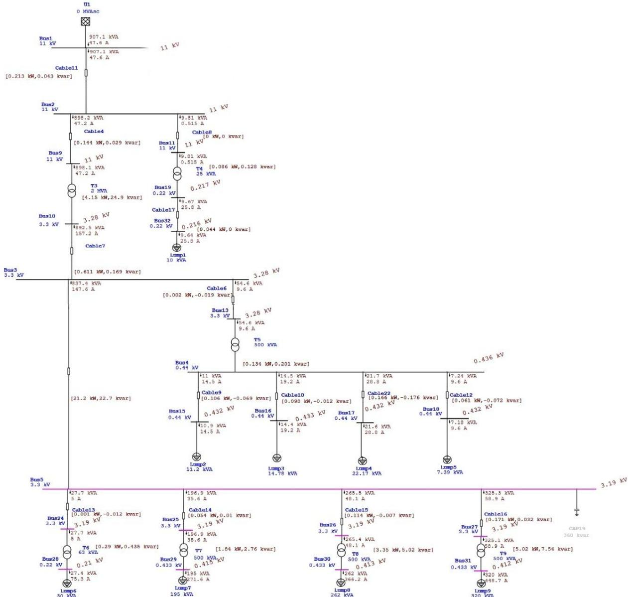
Fig.2 Simulated scheme of substation without capacitor bank in ETAP
