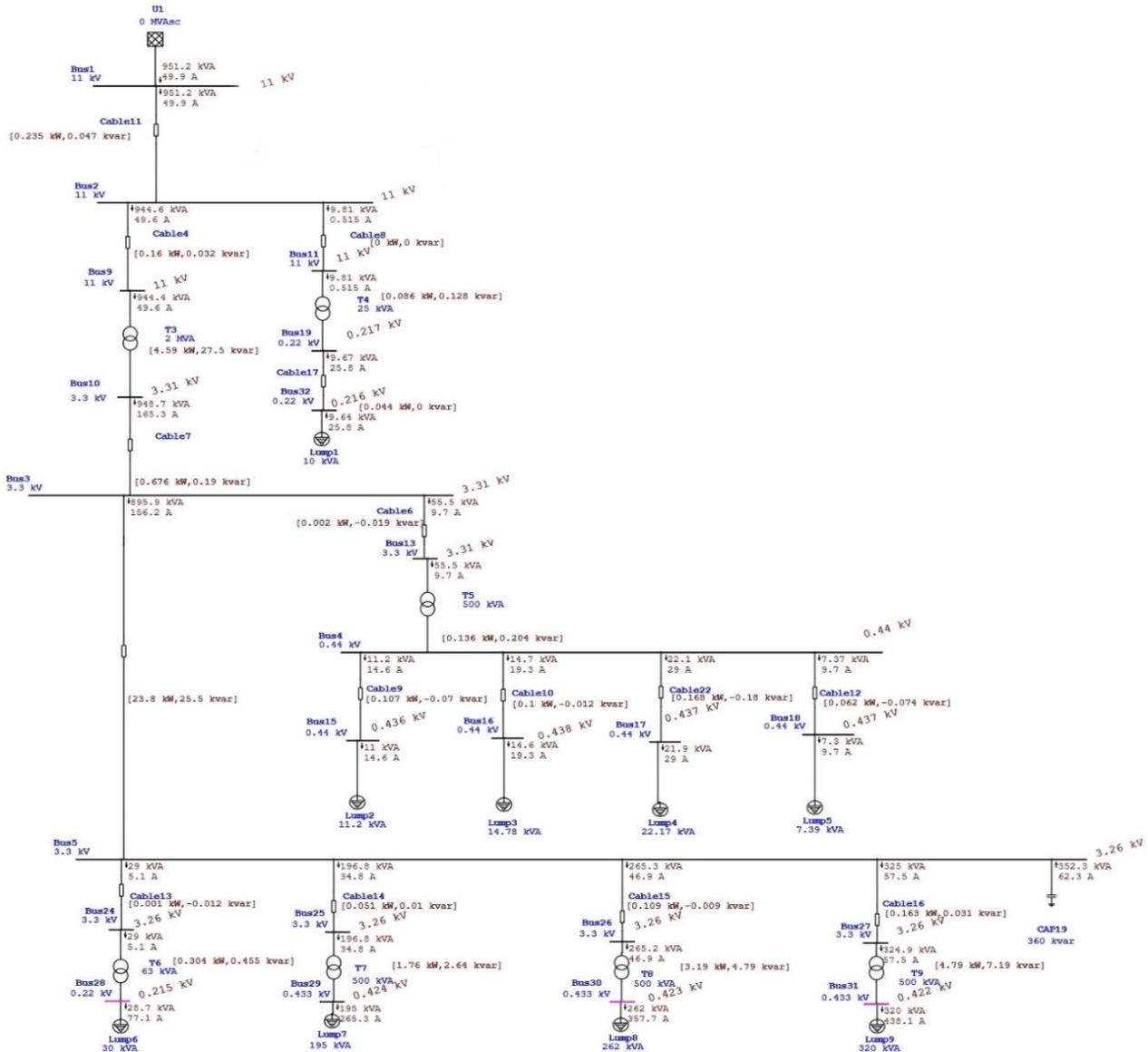
Fig.3 Simulated scheme of substation with capacitor bank in ETAP
