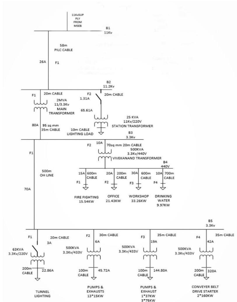
Fig. 1: Single line diagram of substation
