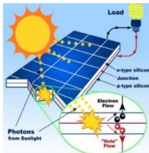
Figure 2: Working Solar Panel
