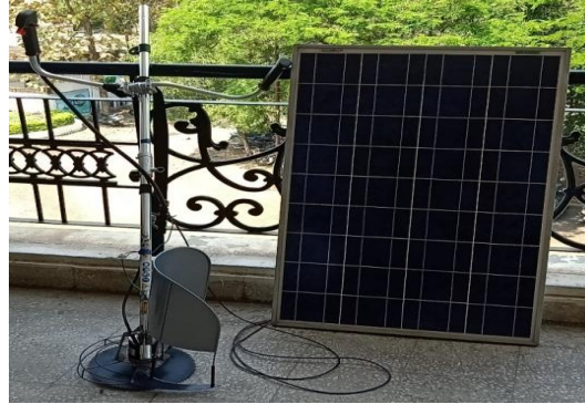
Fig.2 Solar Plate with crop cutter
