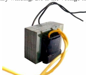
Fig2.3: Transformer (Stepdown 230v/12v)
