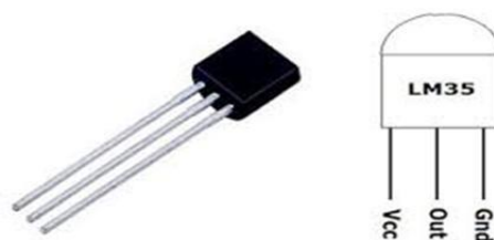
Fig. 2 Pin Diagram of LM35 Temperature sensor
