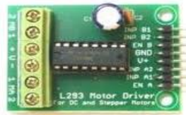
Figure 4: L293 motor driver
