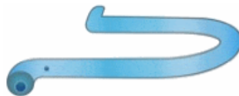
Fig.2. “swinging” is generated by vibrating the tube(s) in which the fluid flows
