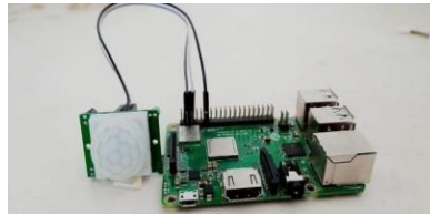
Fig1 PIR sensor and raspberry pi-3 Interface
