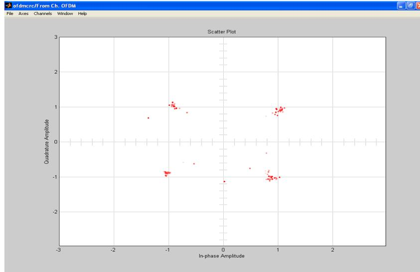
Fig. 5. Scatter Plot of OFDM Received Signal by using QPSK Modulation.
