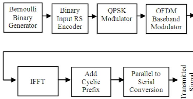
Figure 1. OFDM Transmitter.
