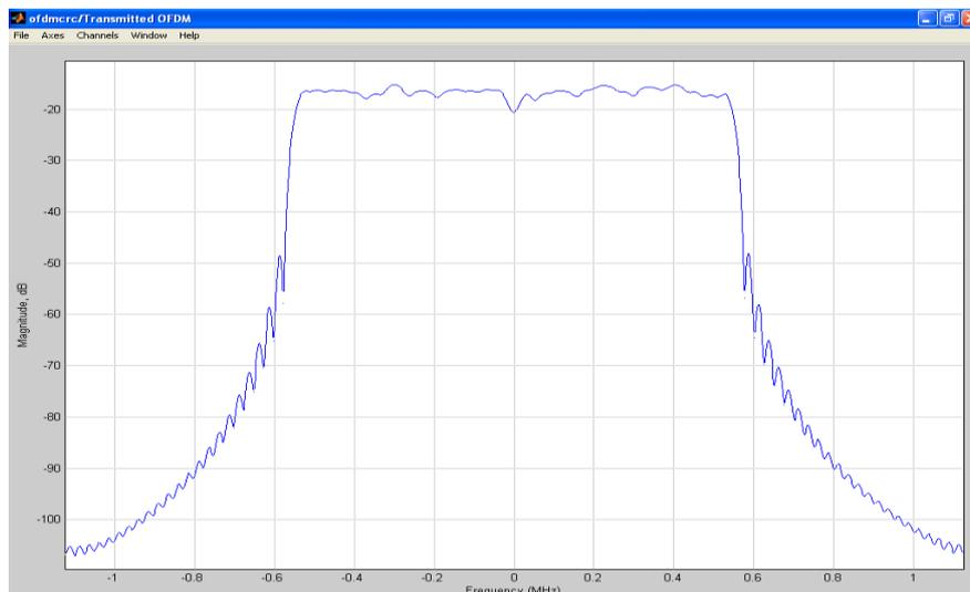
Fig. 3. OFDM Transmitted Signal.
