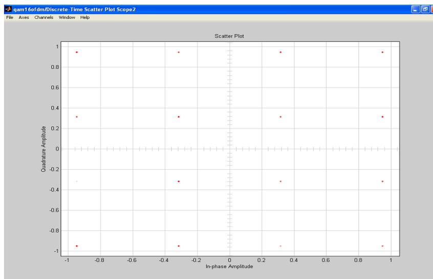
Fig. 7. Scatter Plot of OFDM Received Signal by using 16 – QAM Modulation.
