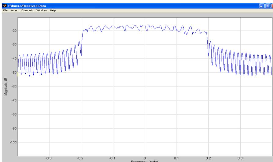
Fig. 4. OFDM Received Signal.
