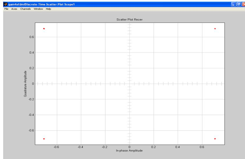
Fig. 6. Scatter Plot of OFDM Received Signal by using 4 – QAM Modulation.
