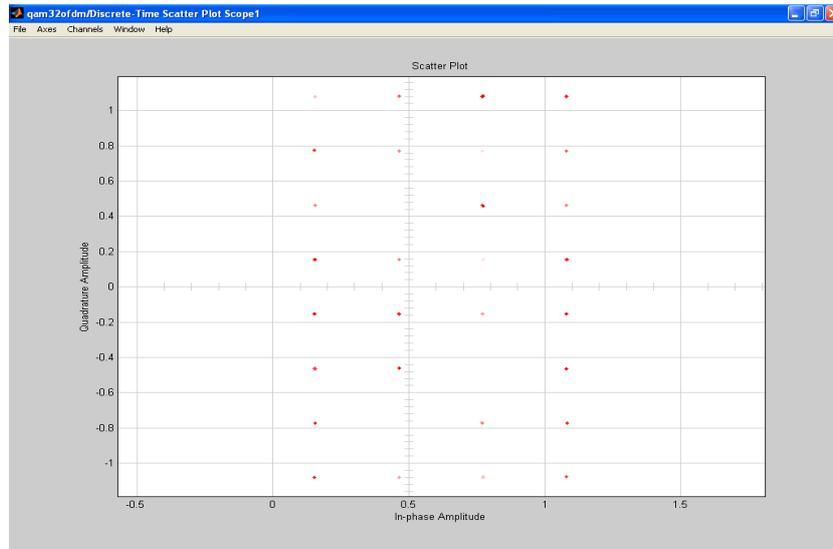
Fig 8. Scatter Plot of OFDM Received Signal by using 32 – QAM Modulation.
