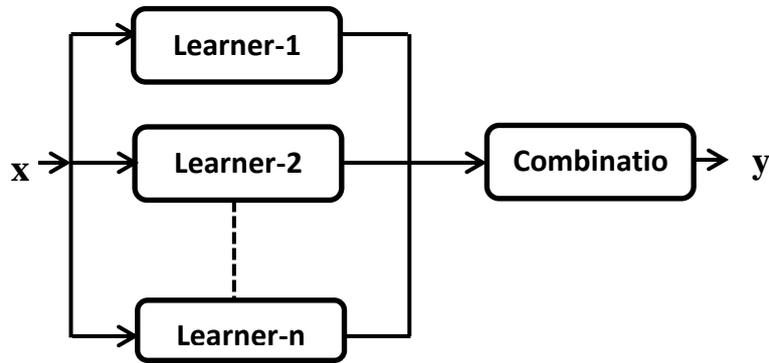
Fig 4: Basic ensemble architecture
