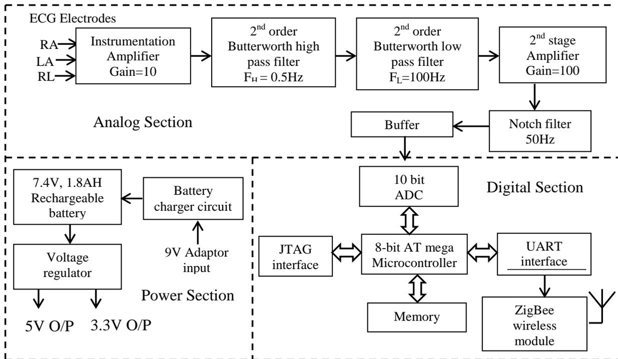
Fig 2: ECG Signal Acquisition Hardware
