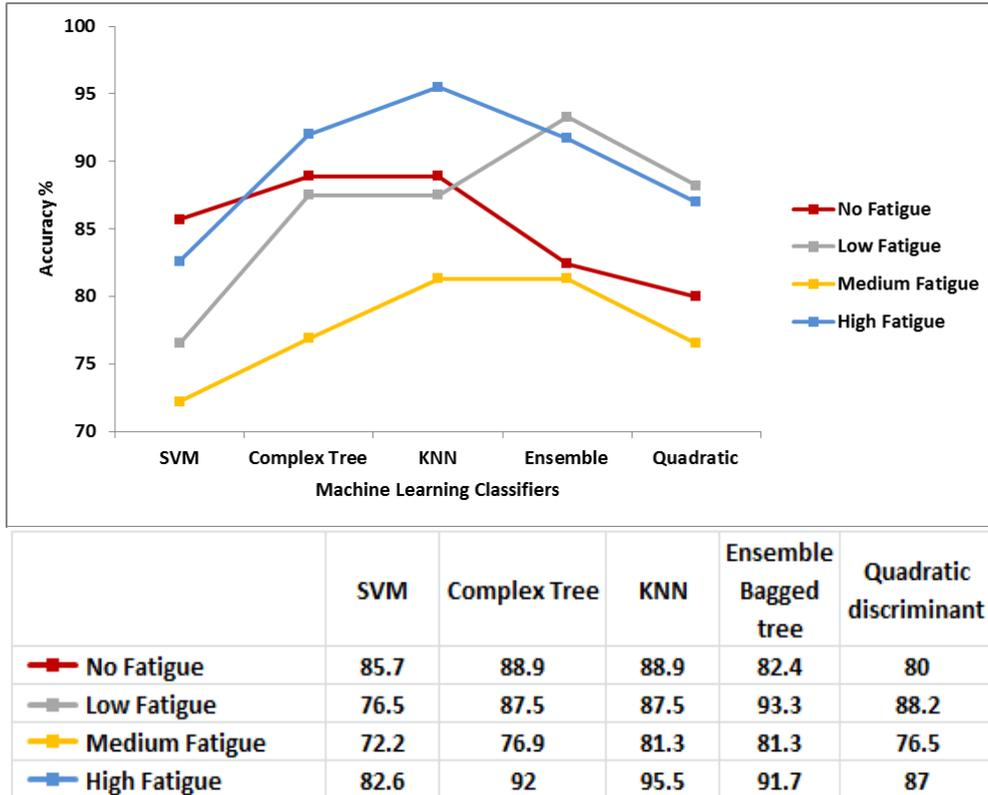
Fig 19: The performance comparison of various machine learning classifiers for No-fatigue, Low, Medium and High fatigue levels
