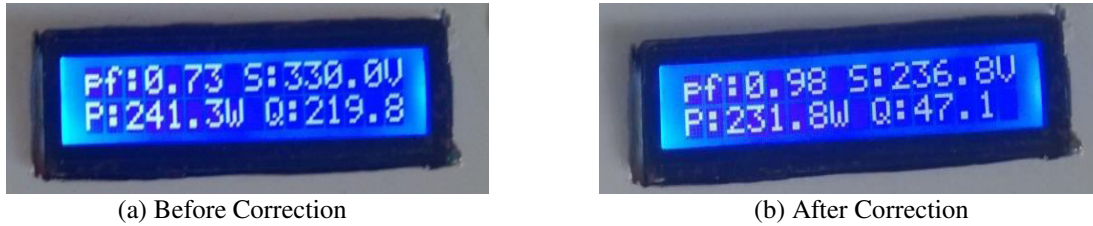
Fig. 8 Result using an AC Blower as Load
