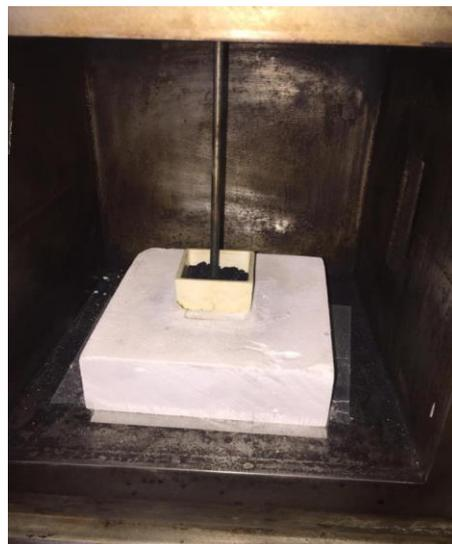
The graphene is placed in alumina crucible K-type thermocouple is being used to measure the temperature. Soaking time is 20 mins under 350 degree Celcius. The resultant graphene will be less in mass as the moisture present in the graphene is evaporated due to heat. To avoid oxidation the sample is processed under Argon Gas.
