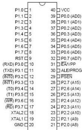
Fig 6.Pin Diagram 89C51 Microcontroller
