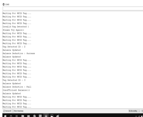
Figure 11. Output of RFID system is displayed on Serial monitor
