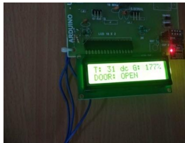
Fig9: Home security system when door is open
