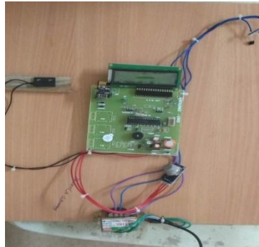
Fig7: Home security system circuit when it is in off condition
