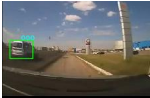
Figure 2. tracking vehicles using mean shift algorithm.
