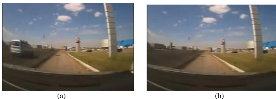
Figure 1. original frame and background: (a) original frame, (b) frame after applying GMM.
