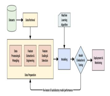
The above figure shows the general steps followed in Prediction project. Where initially data is retrieved. Which is then pre-processed, scaled and selected after extraction and fed into the model to obtain the predictions. The accuracy and predictions can vary based on many factors such as pre-processing techniques, the algorithm used, data been fed into the model as well as the model training procedures.
