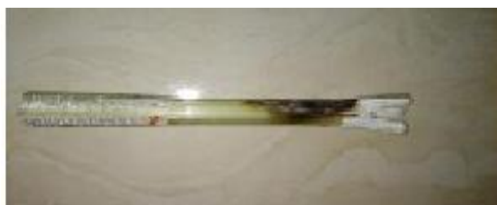
Figure 7: Brittle fracture of FRP rod Sample A
