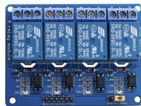
Fig 3: Four Channel Relay
