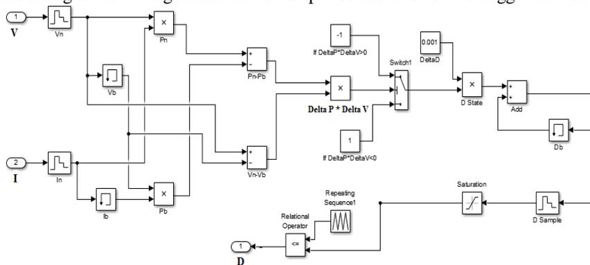
Fig. 11. Modeling of MPPT algorithm
