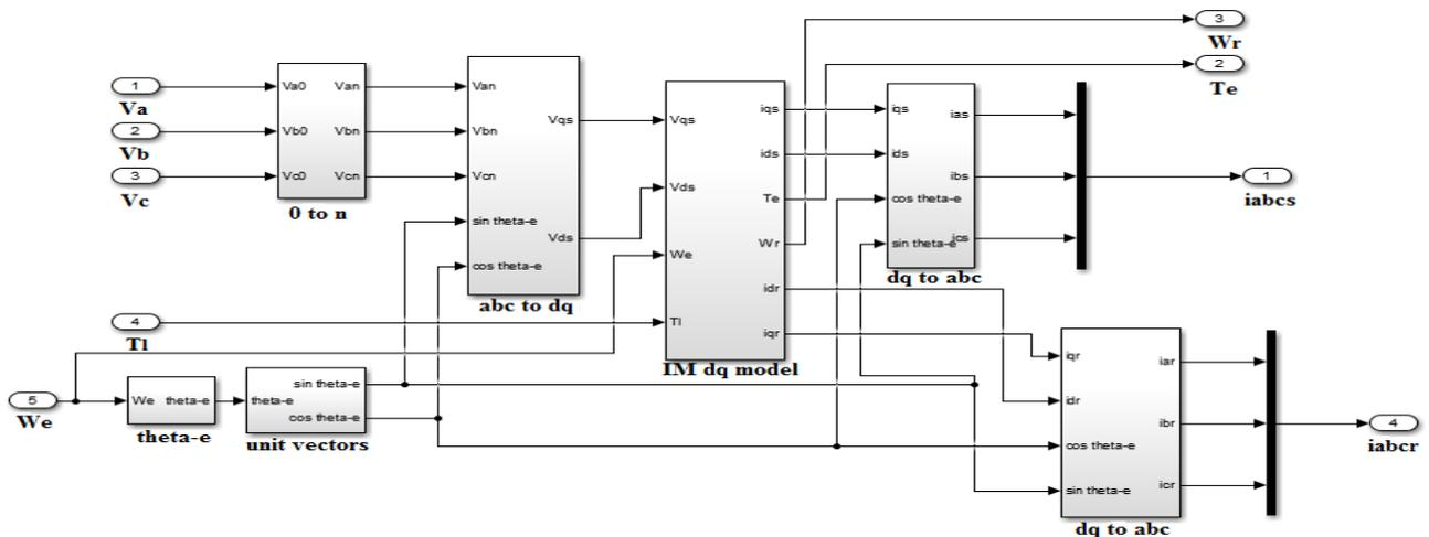
Fig. 3. Modeling of induction motor
