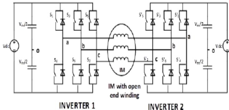
Fig. 2 Open End Winding Induction Motor
