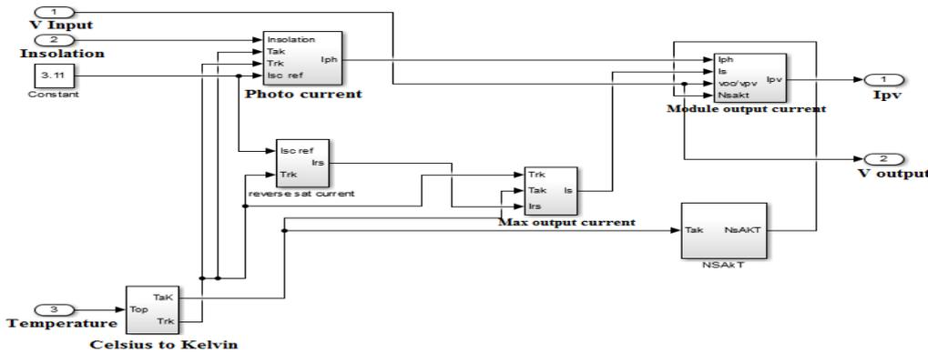
Fig. 8. Modeling of PV system
