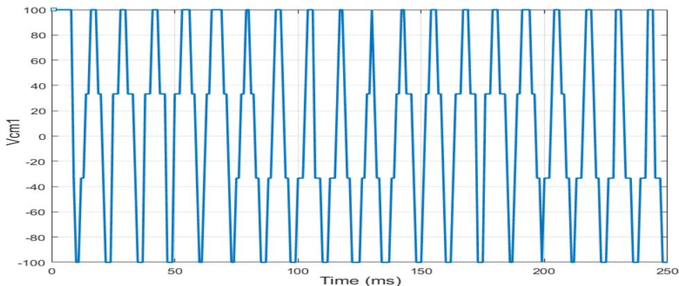
Fig.21. Common mode voltage of inverter 1
