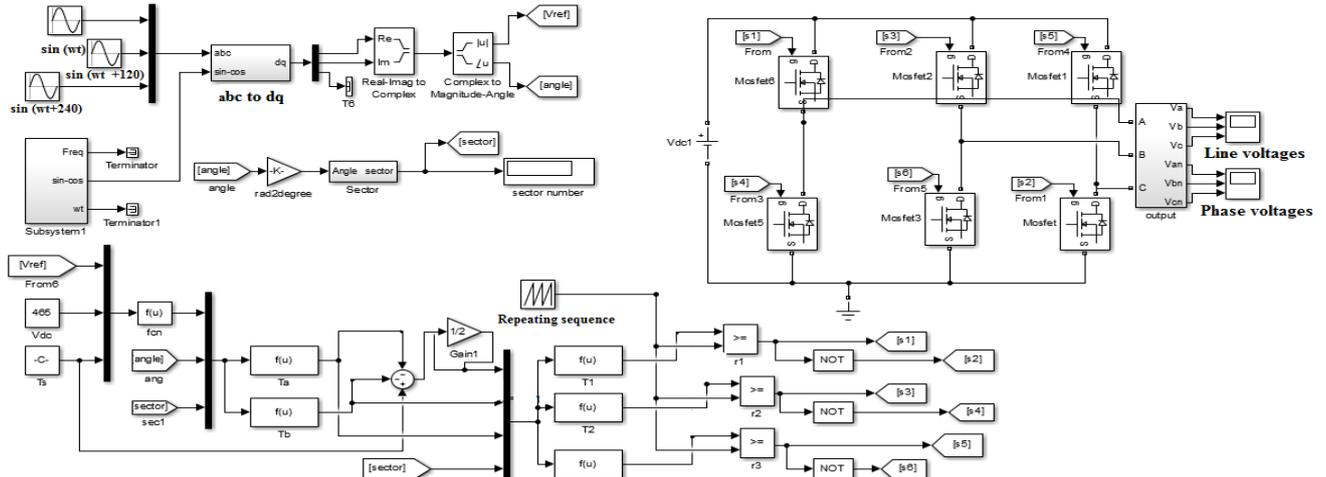
Fig. 15. Modeling inverter and space vector modulation scheme
