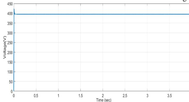
Fig. 13. Output of dickson charge pump voltage multiplier
