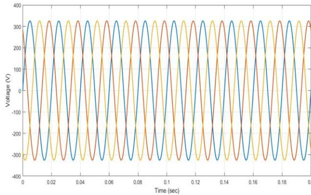
Fig. 4. Input voltage of induction motor
