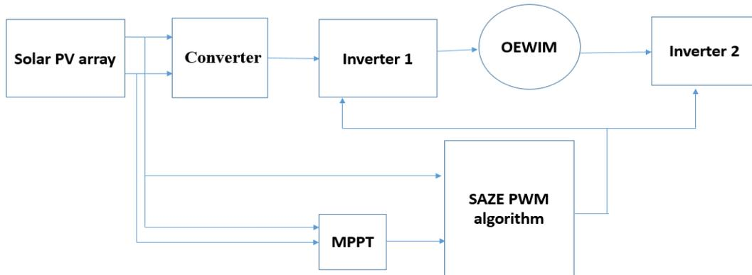
Fig. 1 Block Diagram of Control Algorithms of OEWIM
