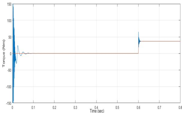
Fig. 6. Torque characteristics of induction motor
