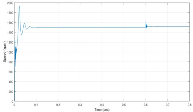
Fig. 7. Speed characteristics of induction motor
