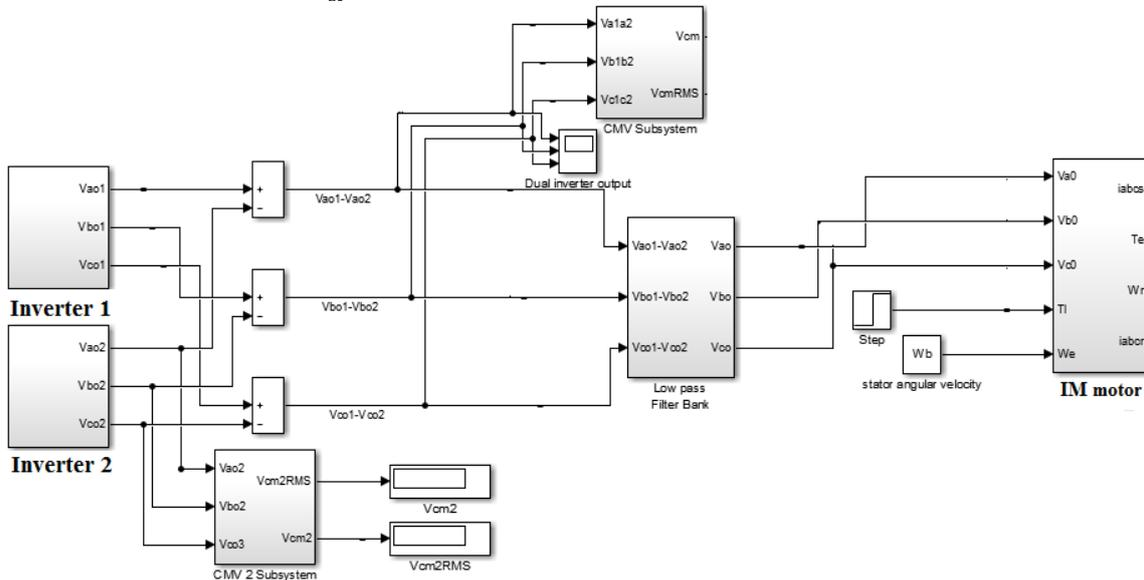
Fig. 14. Modeling of open end winding induction motor
