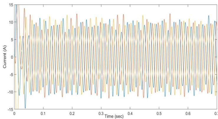
Fig. 18. Output current of open end winding induction motor
