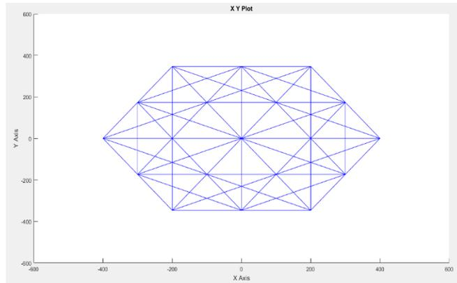
Fig. 16. Space vector of dual inverters
