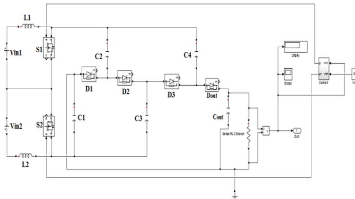
Fig. 12. Dickson charge pump voltage multiplier
