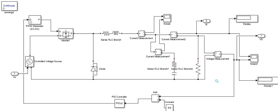
Fig 5: Model of Buck Converter
