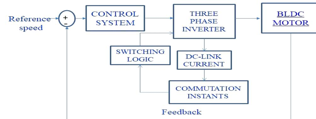
Fig 1: Block diagram representing self-compensation technique
