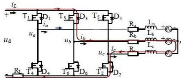
Fig 3: Current circuit after commutation from T<sub>1</sub> to T<sub>3</sub>
