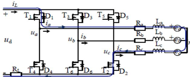
Fig 2: Current circuit before commutation T<sub>1</sub> to T<sub>3</sub>
