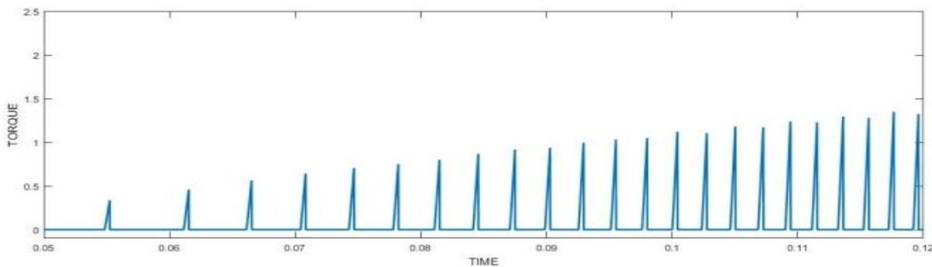
Fig 14: Torque ripple after compensation Vs Time
