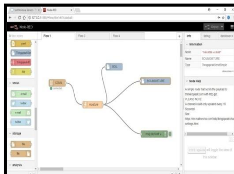
Fig. 9: Node-Red Application for Moisture Sensing
