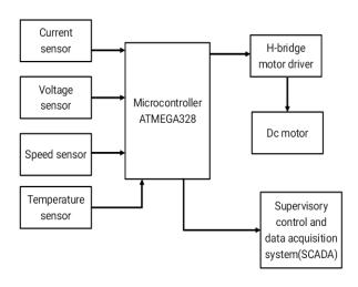
Now DC drive run the DC motor at reference speed. Figure2showstheconfigurationoftheoverallSCADAsystem. This system is divided into three stages which are master station, control unit and motor control. The master station communicates with microcontroller through RS-232cable. OmronCOM1HmicrocontrollerisusedasacontrolunittocommunicatewithSCADA.
