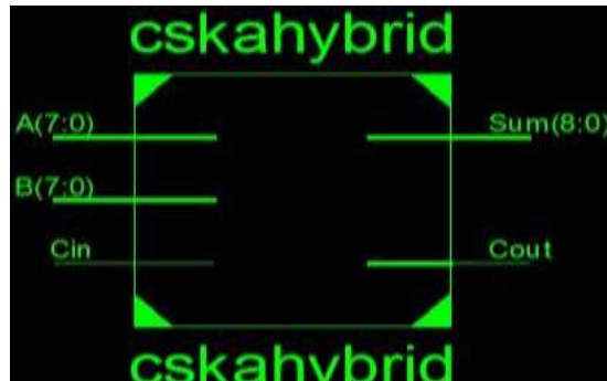
Fig. 8. RTL schematic of Hybrid CSKA
