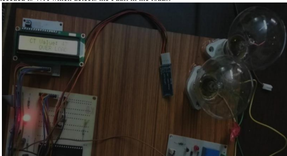
Fig 10: Displays the overload status as Fault detect
