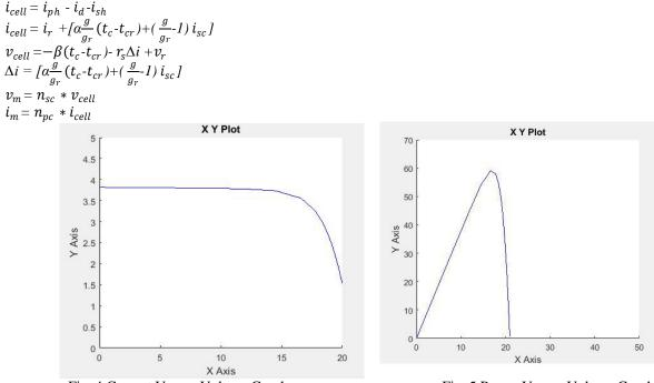
Fig. 4 Current Versus Voltage Graph
