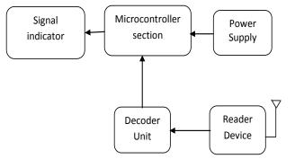
Whenever traffic signal section receives the information about accident, the RF receiver in this section is turned ON to search for ambulance nearing the traffic signal. Whenever the ambulance reaches near to the traffic signal(approximately 100m), the traffic signal will be made to green through RF communication. Thereby the ambulance is recommended to reach the hospital in time.
