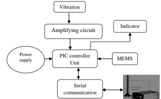
The vehicle unit installed in the vehicle senses the accident and sends the location of the accident to the main server. The main server finds the nearest ambulance to the accident spot and also the shortest path between the ambulance, accident spot and then nearest hospital. The server then sends this path to the ambulance. Also using this information the server controls all the nodes in the path of ambulance and make it ON, which ensures that the ambulance reaches the hospital without delay.
