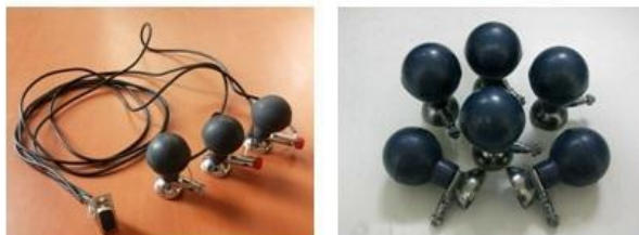
Fig3. Removable Suction Cup Sensors
