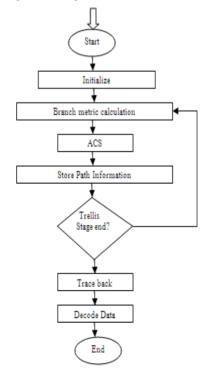
Fig 4: Viterbi decoding Flow Chart
