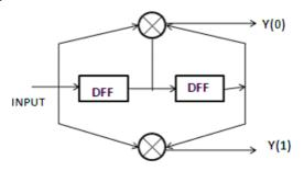
Fig 2. Convolutional encoder
