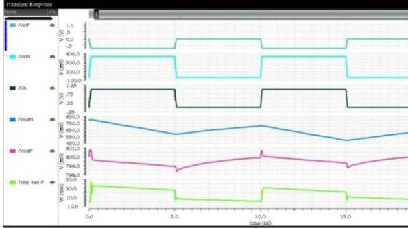
Fig.2. Transient simulations of the conventional dynamic comparator for input voltage difference of  $\Delta V_d = 0.7$  V, and  $V_{DD} = 0.8$  V.
