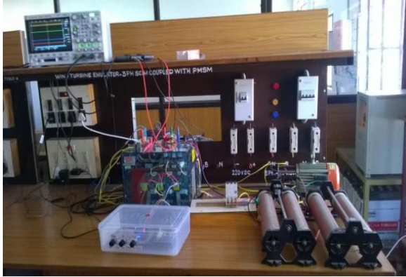
Fig. 18. Hardware setup showing the c2000 launchpad kit, Diode rectifier and load.
