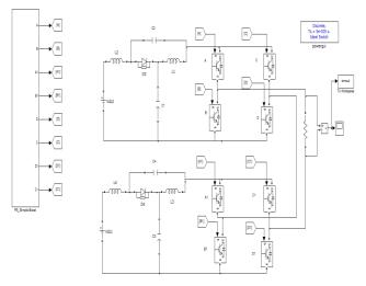
Fig 7. Five level Quasi Z-Source MLI with PSPWM and SBC
