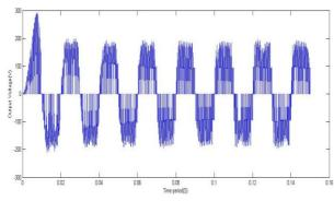
Fig 13.Output voltage of five level QZMLI with PSPWM and CBC
