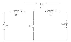
Fig 3.Equivalent circuit of QZSI in active state
