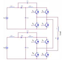
Fig 1. Five - level cascaded H Bridge Quasi Z-Source Inverter www.iiireeice.com 1744
