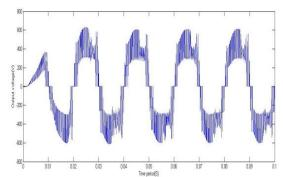
Fig 11.Output voltage of five- level QZMLI with PSPWM and MBC
