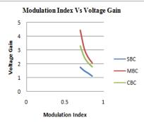
Fig 14 (b) Modulation Index Vs Voltage Gain
