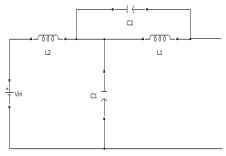
Fig 4. Equivalent circuit of QZSI in zero state
