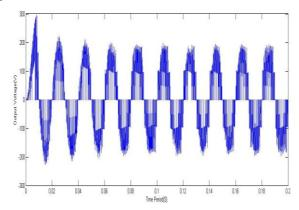
Fig 9.Output voltage of five- level QZMLI with PSPWM and SBC
