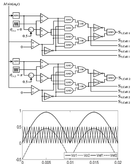
Figure 5: (a) PWM signal generation circuitry (b) Multicarrier phase-shifted PWM for two-cell configuration.
