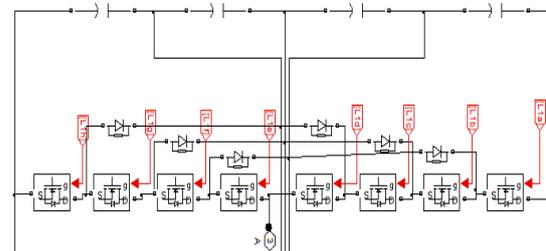
Figure 1: Diode clamped multi-level inverter phase limb
