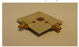
Fig. 2. Fabricated patch antenna [15,16]
