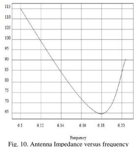
From the above figure antenna impedance is found to be 65 ohm at optimum frequecy 6.18 GHz.
